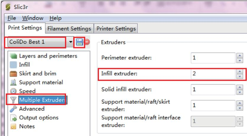
Set the filament of extruder2 to print the infill.
