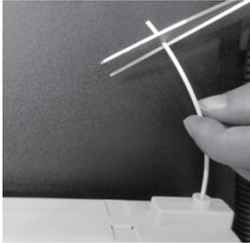
**NOTE:** Do not forcibly pull out the filament from the cartridge in case the filament disorder inside the cartridge.
