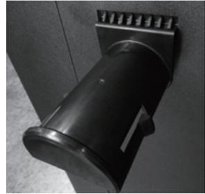
5.6.3 Mount two filament cartridges on the spool holder
