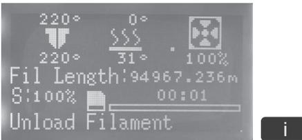
c. When unload ok, finish the filament unloading.
