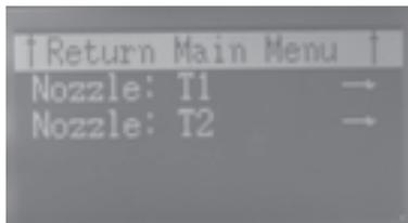
Rotate the knob to select the nozzle you want to take as default nozzle, and its corresponding extruder will be taken as default to work.
