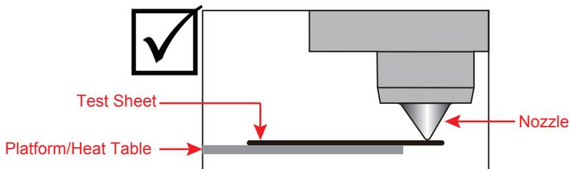
Note: If the calibration standard condition is not met, platform level must be adjusted.
