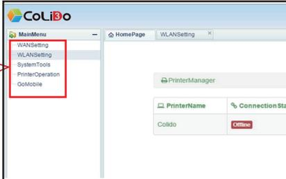
NOTE: When powering off the printer, login to control panel page, under the “System Tools”, click on “ Power off” then switch off the printer.
