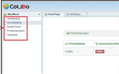
NOTE: When powering off the printer, login to control panel page, under the “System Tools”, click on “ Power off” then switch off the printer.
