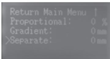
For example, input 2mm and the T1 is the default extruder, then T1 filament (Black PLA) will print 0~2mm, T2 filament (Yellow PLA) print 2~4mm, T1 filament print 4~6mm again, T2 filament print 6~8mm...until finish printing.
