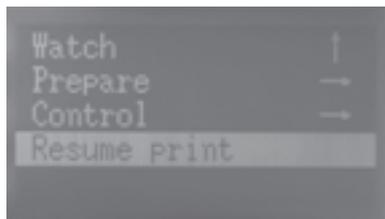
NOTE: When pause printing, the printer head will go to home position and be locked. The nozzle and the platform temperature will keep on.
