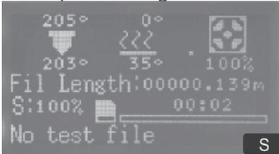
6.4.2 Once the platform temperature reaches the setting temperature, the nozzle will heat up next as picture T.
