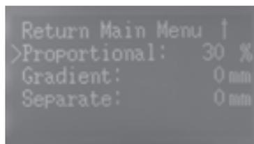
For Example, the default extruder is T1 and input the percentage is 30%, then T1 filament (Yellow PLA ) will be printed 30% and T2 filament (Green PLA) will be printed 70%.
