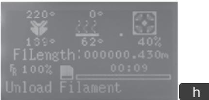
b. Once the temperature reach the setting temperature as below picture g, the default extruder will work to auto unload its filament from the nozzle.
