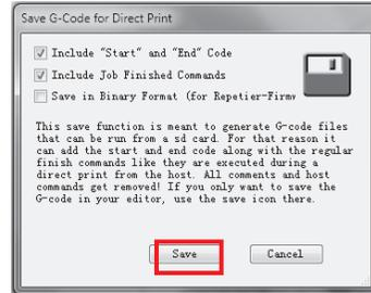
7.4.2 If want to print the file using Repetier-Host, need remove SD Card from the printer.
