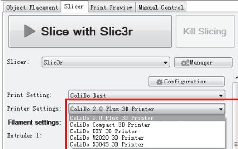
Step 3: Select printer type “CoLiDo X3045 3D Printer”
