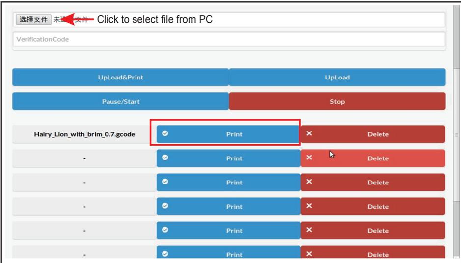
NOTE: The "Pause" and "Stop" function can be use during the printing. During the printer operation might have delay, please wait after click until the page refresh automatically.
