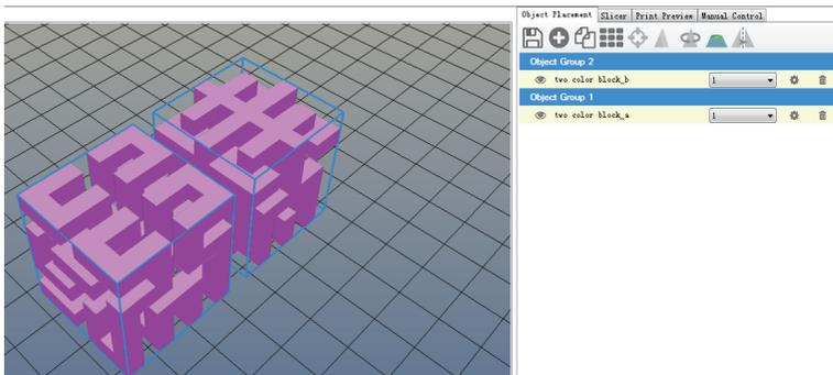
7.7.3 Select file to print use T1 and T2, such as “block\_a” to use extruder T1 and “block\_b” to use extruder T2.
