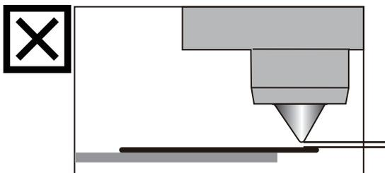
Condition 2: The test sheet is over the nozzle tip.
