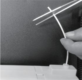
**NOTE:** Do not forcibly pull out the filament from the cartridge in case the filament disorder inside the cartridge.
