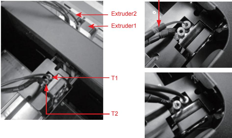
**NOTE:** The filament from Extruder1 must be inserted to T1 as Nozzle1;
