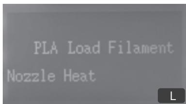
6.3.3 The nozzle will start to heat up as picture M. Once the nozzle actual temperature reach the setting temperature as picture N, the filament will auto load into the nozzle and flow out from the nozzle.
