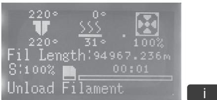
c. When unload ok, finish the filament unloading.
