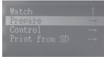
5.5.2.2 Push the knob to go to submenu, rotate the knob to select “Auto Home” and push the knob to confirm. Then, the heat table will be moved up to HOME position.
