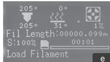
d. Once reach the setting temperature, The default extruder will work to load its filament into the nozzle and flow out. Check the filament flowing condition by refer to 6.3.3.
