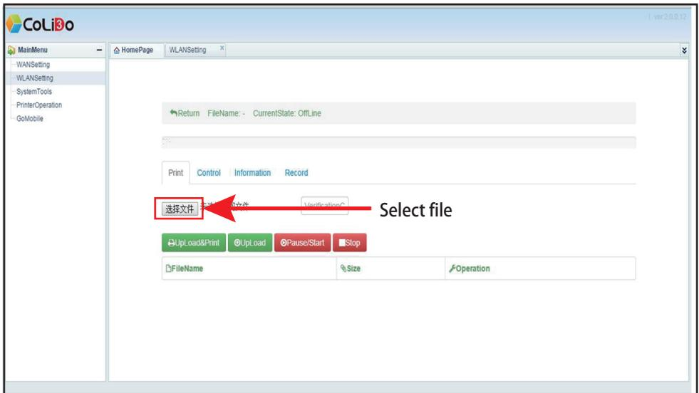
During the print, can use “Pause/Start” and “Stop” button to control. Select "Upload & Print" the model .GCO will show on the list and start print automatically; Select "Upload" the model .Gco will show on the list only. Click "Print" printer will start print the selected .GCO.
