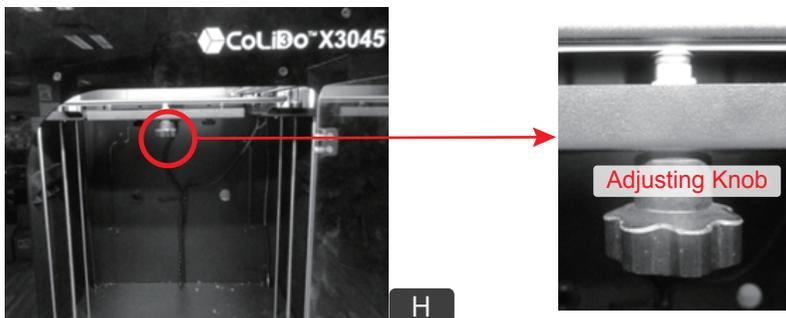
6.2.4 After rotate the adjusting knob to meet the Calibration Standard Condition, rotate the LCD knob to select “Next Step” as picture J, then press the LCD knob to next point to calibrate.
