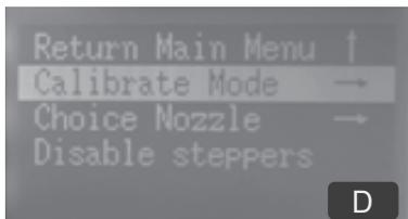
NOTE: “Calibrate Mode”is to guide user to operate the printer and to check if the printer is working well.
